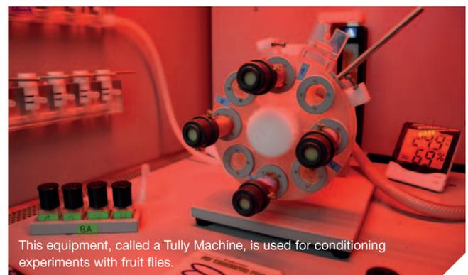
This equipment, called a Tully Machine, is used for conditioning experiments with fruit flies.
