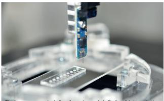
The force sensor probe is finer than a human hair. On the slide beneath the sensor there is a row of PDMS chips, on which the pollen tubes grow.
