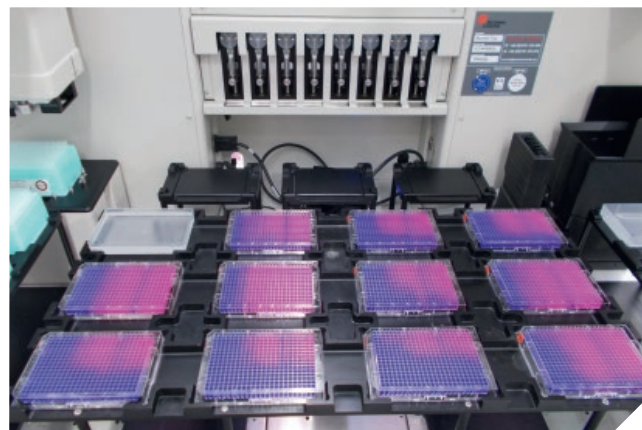
With the help of a pipetting robot, Förster can efficiently test the effectiveness of different combinations and concentrations of antibiotics on different gonorrhea strains. The dye resazurin shows which bacteria are killed (blue), and which survive (pink). Photo: Sunniva Förster
